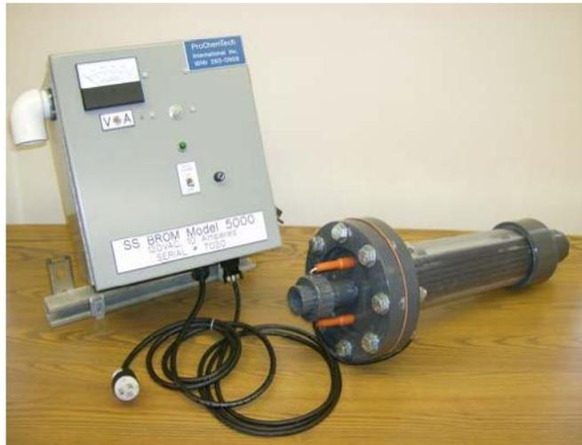
Sufficient bromide ion is provided in the cooling water for operation of the **system** with use of either PCT 6460 B, 6461 B, or 6462 B SofTek<sup>™</sup> water treatment products at the recommended dose levels.
